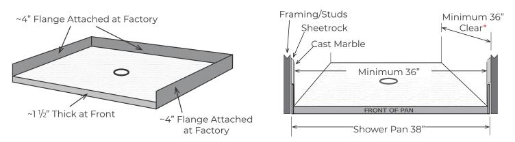
\*Note\* The ADA code requires the finished opening of a transfer pan to measure a minimum of 36" left to right and 36" front to back. The entrance must be flush with the entry floor, just like a roll-in pan.
