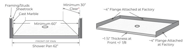
\*Note\* The ADA code requires the finished opening of a roll-in shower pan to measure a minimum of 60" left to right and 30" front to back.
