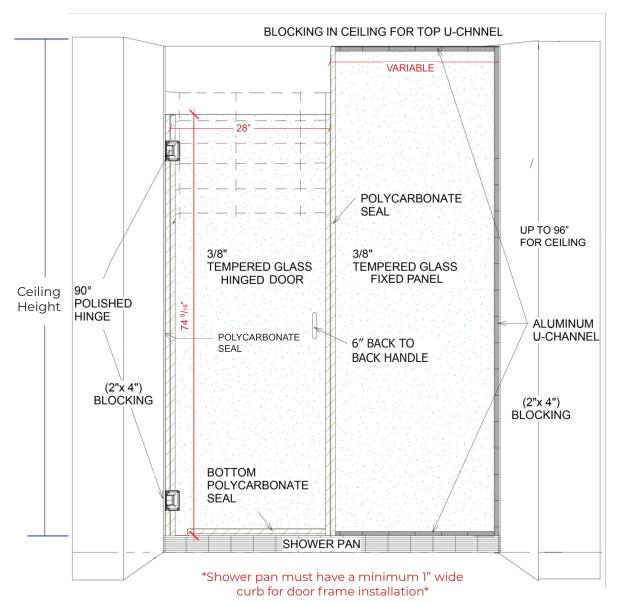
Note: These measurements are based on a standard 60" w x 96" h Enclosure. The MM Hinged heights and widths are variable for the fixed glass panel ONLY, and can be ordered to fit specific project requirements. Please include your project specific w x h measurements when placing your order.
