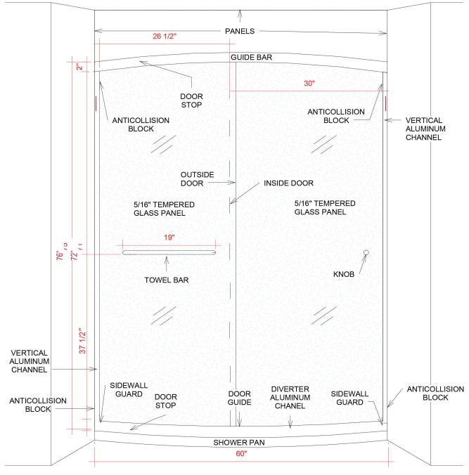
\*Shower pan must have a minimum 3" wide curb for door frame installation centered on the curb.
