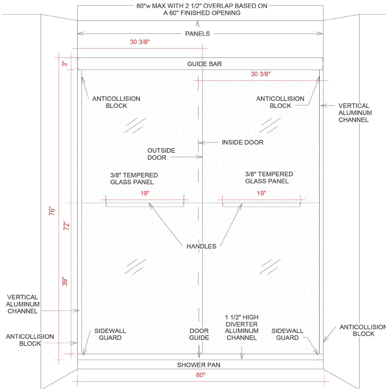
\*Shower pan must have a minimum 3" wide curb for door frame installation\*
