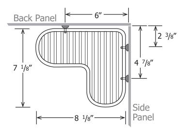
Note: Drill locations in dish may vary so check each dish before drilling. Add a daub of 100% silicone into screw holes under chrome screw cap. Mounting hardware is included.
