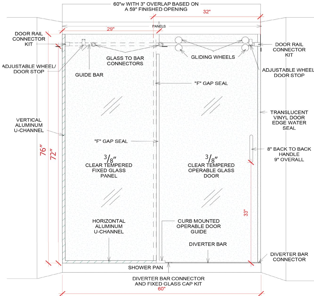
\*Shower pan must have a minimum 3" wide curb for door frame installation\*
