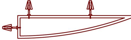
5. Apply 100% silicone to the entire back of the foot rest, using a minimum ¼" bead of silicone. **This step cannot be skipped or avoided, as the silicone adhesive is a necessary product in the installation of the foot rest as the truss head screws are not designed to be a stand alone installation product.**
