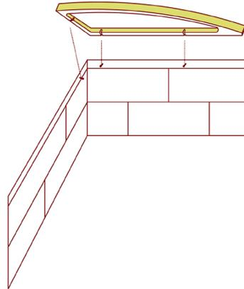
6. Using a # 2 Phillips head screwdriver, tighten the truss head screws as tightly as possible. You will hear creaking noises when the screw is tight against the support of the foot rest. **A right-angle screwdriver will make it easier to turn the screws. A ratcheting right-angle screw driver is optimal for this installation.**
