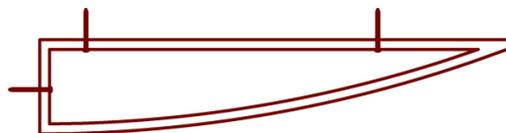
4. Apply 100% silicone to the entire back of the foot rest, using a minimum ¼" bead of silicone. ***This step cannot be skipped or avoided, as the silicone adhesive is a necessary product in the installation of the foot rest as the truss head screws are not designed to be a stand alone installation product.***
