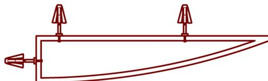
5. Apply 100% silicone to the entire back of the foot rest, using a minimum ¼” bead of silicone. **This step cannot be skipped or avoided, as the silicone adhesive is a necessary product in the installation of the foot rest as the truss head screws are not designed to be a stand alone installation product.**
