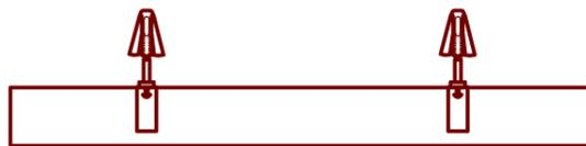
6. Apply 100% silicone to the entire back of the ledge and into the hole that will receive the mounting hardware.
