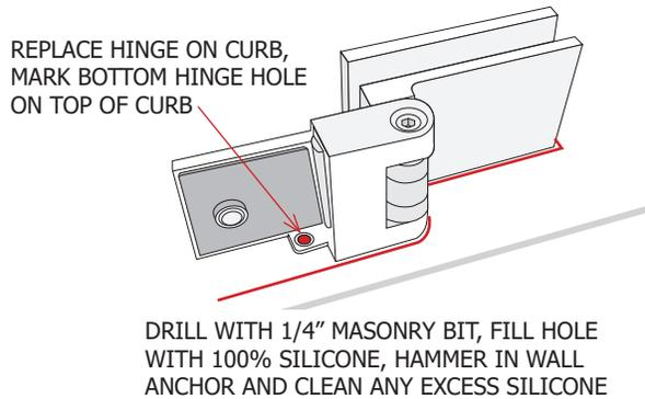
Next, Screw the Bottom Hinge onto the Shower Pan Curb. Then, Fill the bottom corner of the Fixed Glass Panel U Channel and around the base of the U Channel where it meets the Shower Pan with 100% Silicone. Next, Place the Fixed Glass Panel into the Bottom Hinge and the U Channel and Re-assemble the Bottom Hinge making sure the Fixed Glass Panel is Level. Clean any excess silicone.
