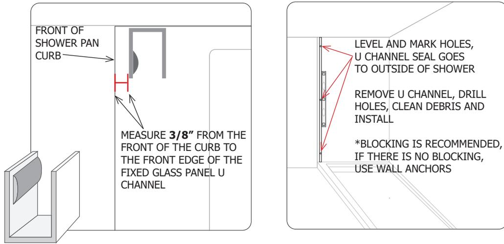
Next, remove all of the plastic protective coating on the Bottom Hinge, install the Bottom Hinge onto the Fixed Glass Panel and Place it into the Wall U Channel. Door Hinge goes to the inside of the shower. Adjust so that the Fixed Glass Panel is Level.
