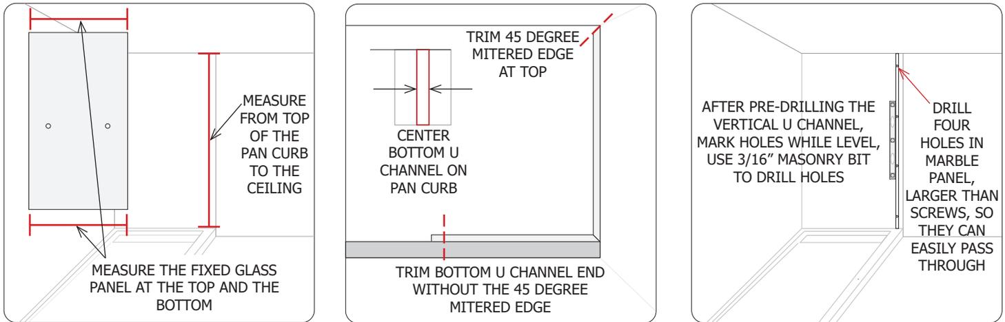
Measure the Top of the FIXED GLASS PANEL. Trim the TOP U CHANNEL like the BOTTOM U CHANNEL. Pre-drill and Countersink 3 holes in the Top and Bottom U Channels.
