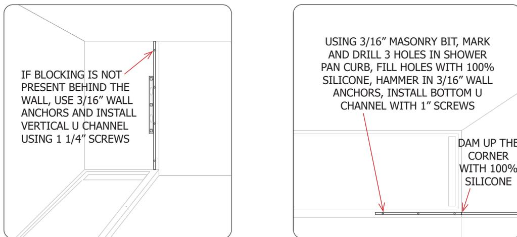
After installing the VERTICAL and BOTTOM U CHANNELS, dam up the Bottom Corner Seam with 100% Silicone.
