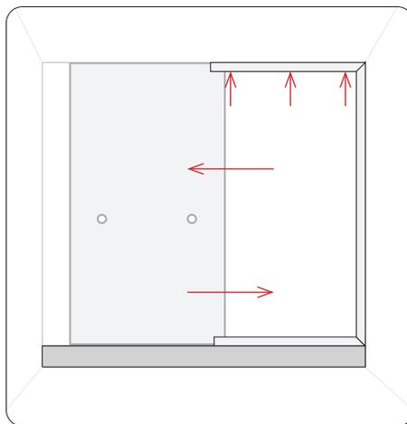
CAREFULLY SLIDE GLASS PANEL OUT OF THE WAY OF THE SCREW HOLES IN THE TOP U CHANNEL, SCREW TOP U CHANNEL INTO PLACE USING 3/16" WALL ANCHORS IF BLOCKING IS NOT PRESENT.
