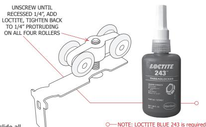
After applying LOCTITE to the ROLLER SCREWS, slide all four ROLLERS into the HEADER as shown below, with the SHOWER DOOR CONNECTING TABS positioned to the outside.
