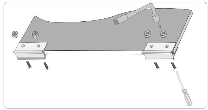
Side view of the glass door after the glass bracket is installed.
