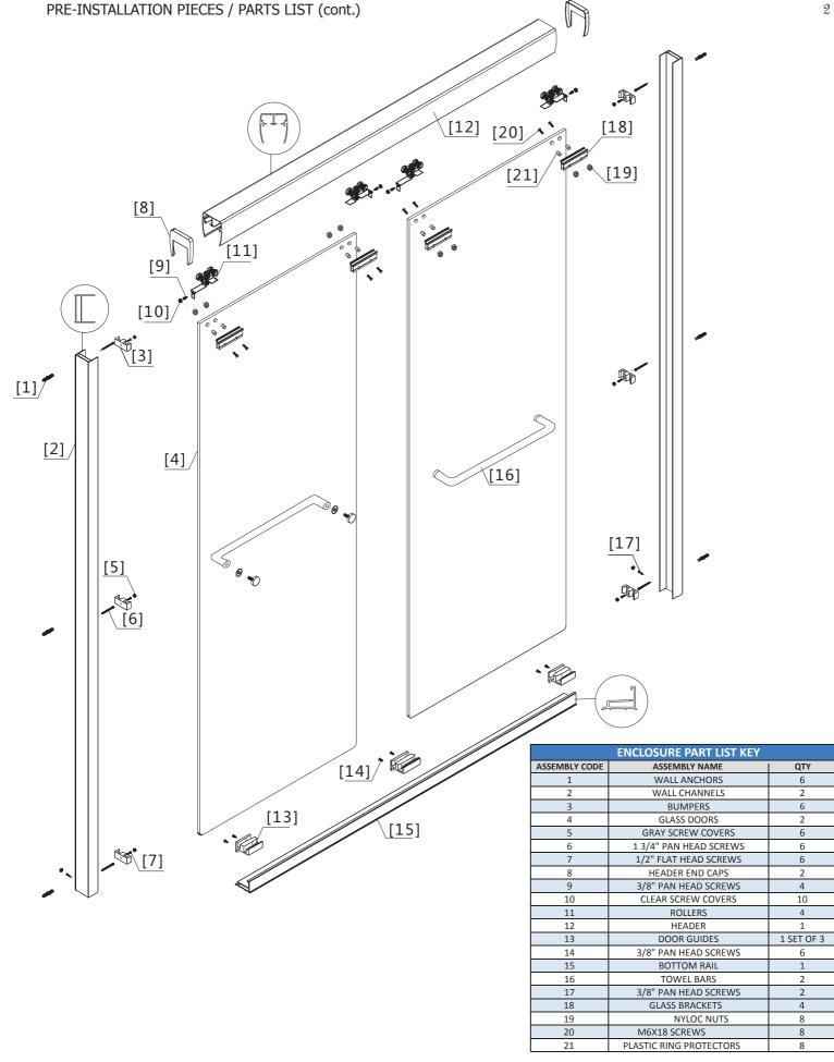
These instructions are to be followed assuming the Shower Pan is level and the Walls are plumb. After you have confirmed that all of the remaining parts and pieces are present, you are ready to begin by installing the BOTTOM RAIL first. Start by removing the three DOOR GUIDES from the BOTTOM RAIL in their Left, Center and Right designated locations. They will be re-installed near the end of the enclosure assembly completion. Be sure to keep up with the screws.
