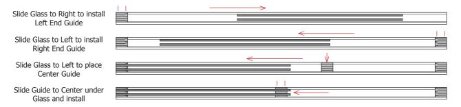
After you have installed the Door Guides, you will need to adjust the Glass Doors for proper alignment. You can adjust the doors Vertically by adjusting the SCREWS in the ROLLERS on each end of the doors. You make any adjustments by carefully sliding out the ROLLER from the Glass Door Bracket just enough to access the screw. You can raise the door by Tightening the Screw or Lower it by Loosening the Screw.
