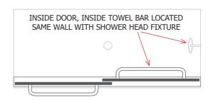
Install the TOWEL BARS in the pre-cut holes in the GLASS DOORS. Be sure to tighten the TOWEL BAR ENDS with a 3/32" ALLEN WRENCH - the hole used for tightening is not a Set Screw, use the hole to rotate the end until extremely tight.
