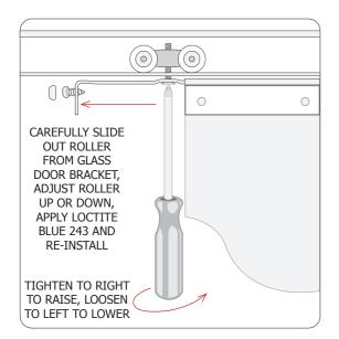
Proper alignment for the Shower Doors would be Flush to the Bumpers in the Side Vertical Wall Channels, hanging Level, above the Door Guides in the Bottom Rail without any interference when operating back and forth.
