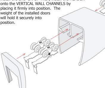
Once the Header is in place, slide the Rollers towards outside edges to make room for the Shower Doors. You will want to install the Outside Edge Shower Door first. You will use four 3/8" Pan Head Screws to connect the Rollers to the Glass Door Brackets, using LOCTITE BLUE 243 threadlocker when installing. The two Rollers on each end will allow for adjustment to align the heights of the Shower Doors properly.
