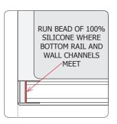
The DOOR GUIDES interlock into the Bottom Rail. Slide them back into the Bottom Rail as they were disassembled at the beginning of these instructions. Start with the two END DOOR GUIDES (refer to following page.)
