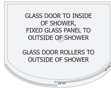
TOP ROLLERS ON THE GLASS DOOR TO THE OUTSIDE OF THE SHOWER, THE ADJUSTMENT SCREW GOES TO THE BOTTOM FOR ACCESSIBILITY
