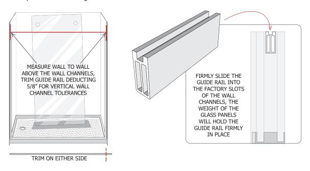
To install the GLASS PANELS, begin with the BACK GLASS PANEL that is already placed inside the Shower. Carefully align the bottom of the GLASS PANEL into the CENTER DOOR GUIDE located on the WATER GUARD as you hang the ROLLERS onto the GUIDE RAIL. Make sure the ROLLERS are facing out of the Shower on the Inside Panel.
