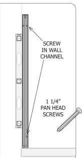
CLEAN DEBRIS AND SHAVINGS, PLACE WALL CHANNEL AND SCREW INTO PLACE
