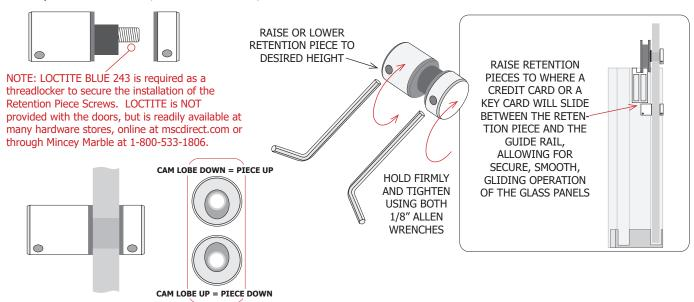
You are now ready to install the FRONT GLASS PANEL. Carefully align the bottom of the GLASS PANEL into the CENTER DOOR GUIDE located on the WATER GUARD as you hang the ROLLERS onto the GUIDE RAIL. Next, follow the same instructions as the Back Glass Panel and adjust the height of the Glass Panel with the Rollers to the desired position and install the Retention Pieces. Then, you can proceed to installing the TOWEL BARS.
