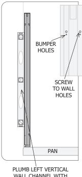
PLUMB LEFT VERTICAL WALL CHANNEL WITH LEVEL, MARK LARGER HOLE LOCATIONS AND REMOVE
