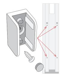
Next you will prepare to install the GLASS PANELS. Start by disassembling the ROLLERS and installing them onto the GLASS PANELS.
