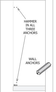
REMOVE WALL CHANNEL, DRILL HOLES WITH 5/16" MASONRY BIT, HAMMER IN WALL ANCHORS
